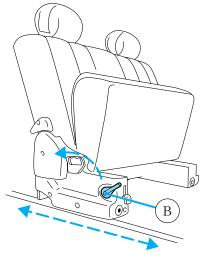
After sliding the seat, check to ensure that both sides of the seat are locked in position. This must be done before the vehicle is put into motion in order to prevent unintended movement of the seat.
